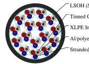
LSOH (SHF1) Outer Sheath Tinned Copper Drain Wire XLPE Insulation Al/polyester Tape Screen
